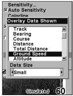
Overlay Data command on the Sonar Menu, at left. Overlay Data Shown selection menu, right. In this example, we scrolled down the data list to highlight "Ground Speed."
